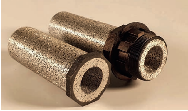
Fig. 3. When functionalizing components made of porous aluminum, the plastic melt enters the surface layer.
